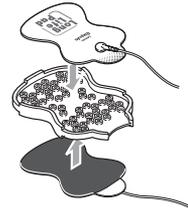
4. Bundle the Electrode Cord and wrap it around the Electrode Holder.
